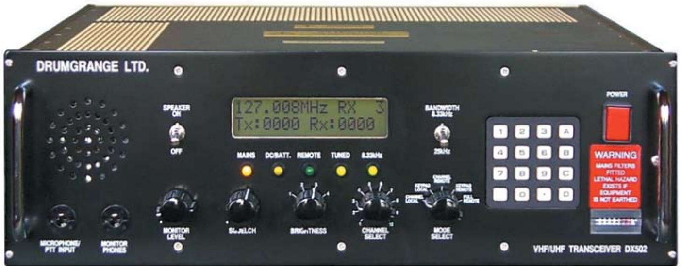
Drumgrange DX502 Transceiver (over 250 units in service with the Royal Air Force)
